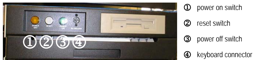
Figure 3-4. Power Control Panel
