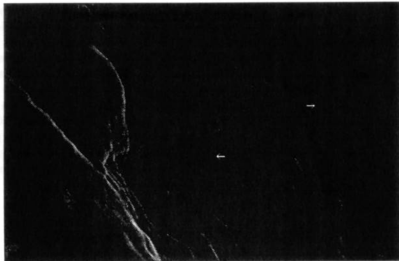
Figure 3.4 Loss of Contrast Due to Charging
