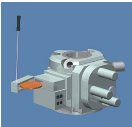
Type I stage and type I airlock
