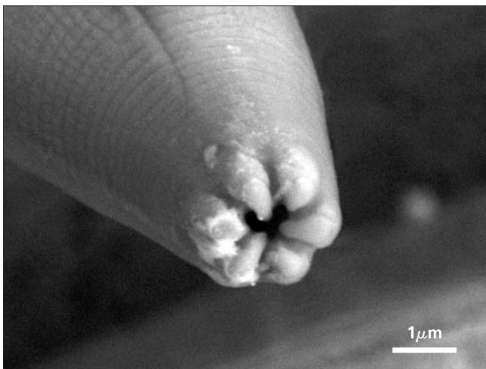
Nematode, Chemically fixed, dehydrated, replaced with t-butyl alcohol, freeze dried in LVSEM Specimen courtesy of Prof. E. Kondo, Saga University, Japan.
