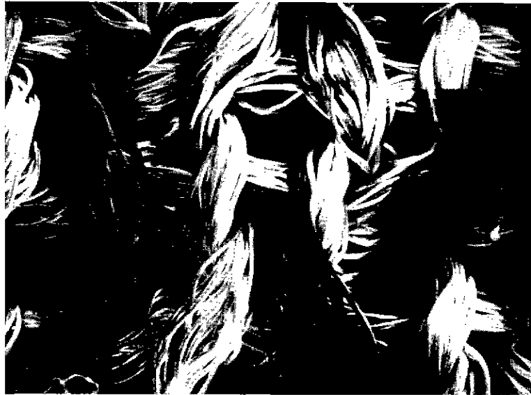
Fig. 1.31 Abnormal contrast due to charging Specimen: Synthetic fibers
