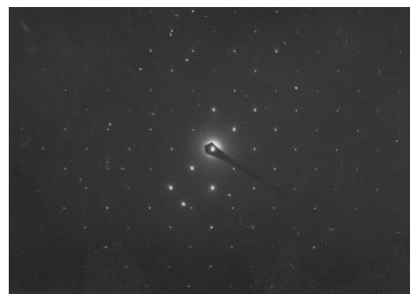
b: Microbeam diffraction pattern
