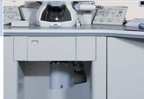
GATAN EELS spectrometer is installed.
