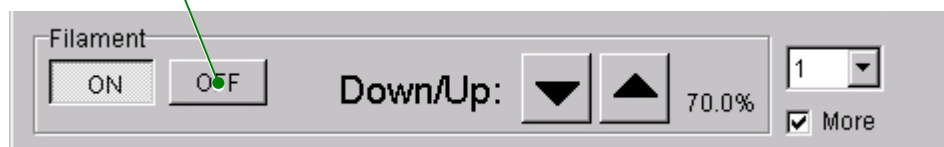
Fig. 5.16 High Voltage Control window(Turning off the filament)
