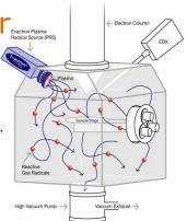
In the Evactron Plasma, oxygen radicals are created. Then, they flow through the chamber from the Evactron Plasma to the pump port. The radicals chemically etch *inside the chamber* any hydrocarbon contamination they encounter. The reaction products are CO,  $CO_2$ , and  $H_2O$ , which are then pumped out of the system.
