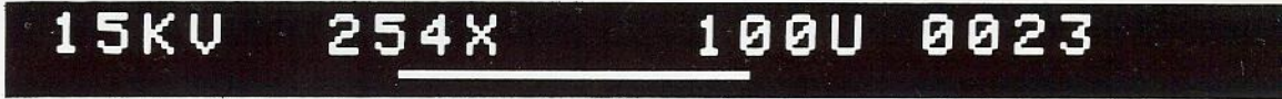
kV, magnification, micron bar with value and 4 digit automatically sequencing serial number are all printed automatically on every micrograph.
