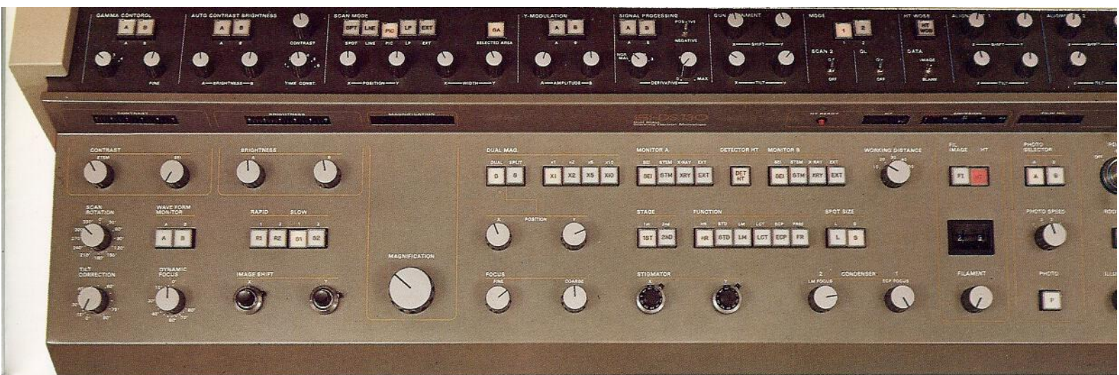
Note the console design for ease of use. Non-routine operation controls (top) are usually left covered.
