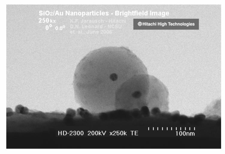
Instrument : Hitachi 200 kV dedicated STEM, HD-2300 Sample rotation: 0 to 360°
