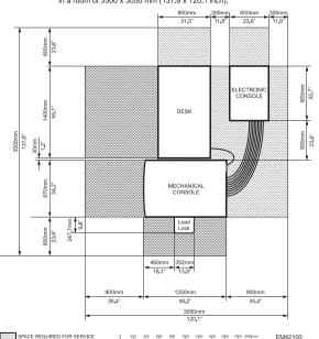
If you position the electronic console behind the desk, you can place the system in a room of 3500 x 3050 mm (137.8 x 120.1 inch).
