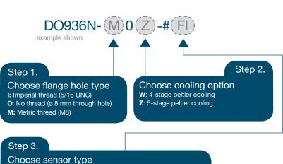
BN: Back Illuminated CCD, with no AR coating FI: Front Illuminated CCD
